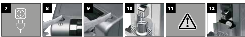
7 Insert the plug. 8 Press the ON button (B) for one second. 9 Press the coffee button (A). 10 Wait for the water to come out of the distributor (E) and leave it running for two minutes. 11 The flow will not stop automatically. To stop it push the button (A). 12 Retrieve the orange capsule which must be preserved for subsequent washing.
