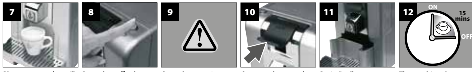
7 Place a cup on the grill. 8 Press the coffee button (A). The flow will not stop automatically. To stop it press the button (A). 9 Once the quantity desired has been reached, press the button (A). 10 Once you have made a coffee always expel the capsule. Capsules are automatically expelled by opening the hatch. 11 Periodically empty and rinse the basket (F) and the tray (H). 12 The machine shuts off automatically in 15 mins. after the brewing of the last coffee, to save energy.
